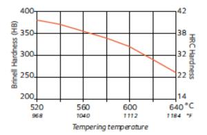
NOTE: Complicated shapes require accurate control of steel temperature uniformity and sufficient holding times to limit stresses and prevent cracking.
