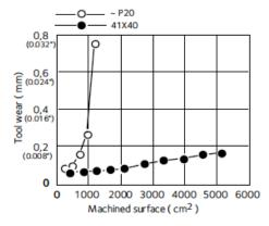
NOTE: Tool wear in fine milling with TiCN coated carbide tools
