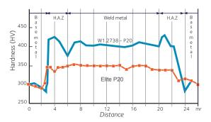
NOTE: Comparison of hardness uniformity through out welded zone for Elite P2O and W1.2738-P2O.
