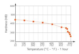
Elite P20 is adapted for surface treatments like nitriding (ionic or gaseous), PVD coatings, providing that those processes do not request heating higher than 550°C (1020°F).
